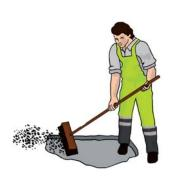
Sweep the pothole clean and remove any water. If necessary, straighten the edges to be perpendicular. First fill deep potholes with gravel and compact. Apply a 10–40 mm layer of the asphalt repair compound, depending on the thickness of the asphalt. Prefilling and compacting the potholes saves a great deal of patching material without compromising the quality or durability of the end result. If necessary, widen cracks before patching them.
